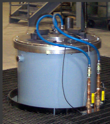
HIP Unit 3 achieves a maximum temperature of 2550°F
